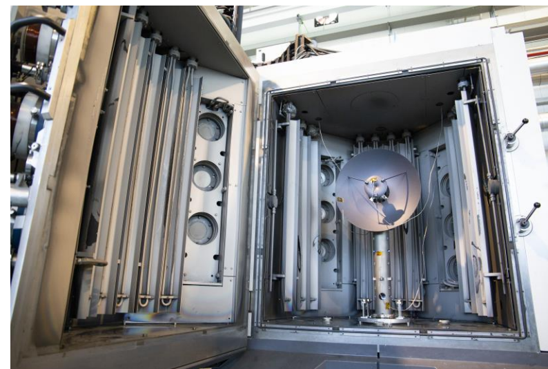
TiC (anti cold-welding) coated antenna for JUICE MISSION
